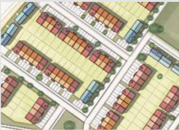
Layout is constrained by the mandatory distance limiting densities to max 32/Ha
