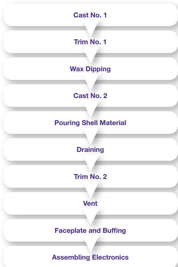
Figure 7: Traditional manufacturing process for hearing aids
