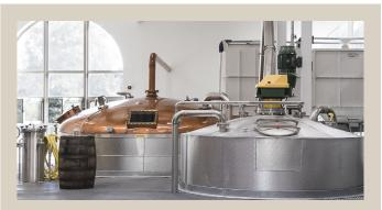
Powerscourt Distillery utilises 100% renewable biogas to make their whiskey and then harnesses the heat from the mashing process using heat exchangers to power the underfloor heating for the Visitor Centre.
